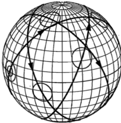
Figure 3.3 – Walker-Delta pattern at i = 65^\circ [16].
